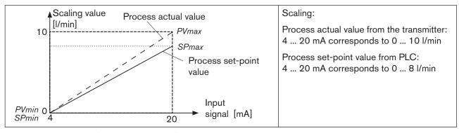
Figure 28: Example of a sensor calibration for signal type 4 - 20 mA
