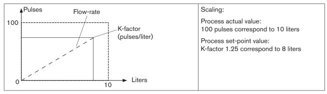
Figure 29: Example of a sensor calibration for frequency signal type
