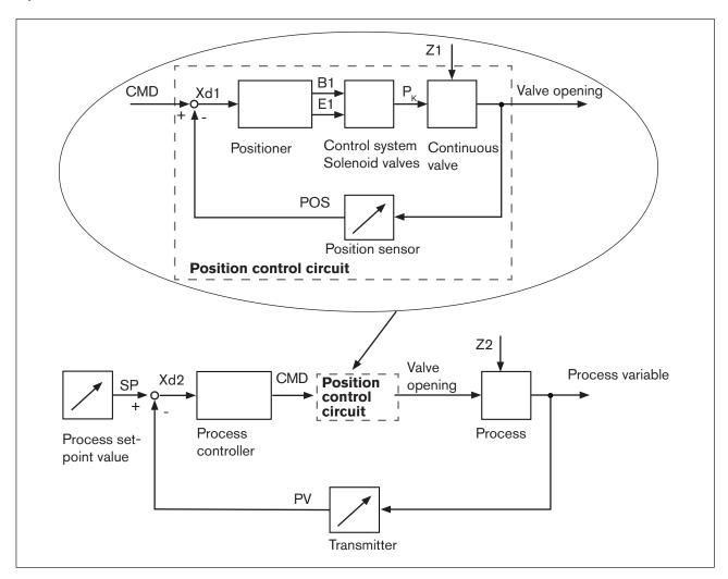
Figure 5: Signal flow plan of process controller
