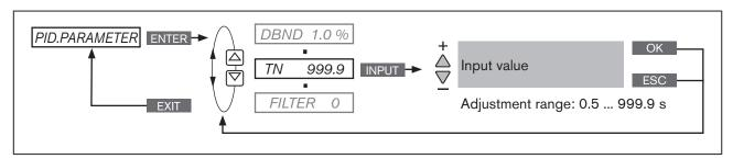
Figure 36: Operating structure TN; reset time
