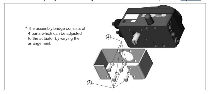
Figure 14: Attach assembly bridge (schematic representation)
