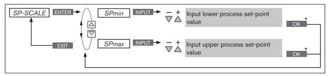
Figure 31: Operating structure SP-SCALE
