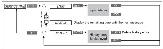
Figure 83: Operating structure SERVICE.TIME
