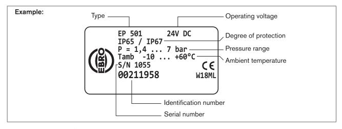
Figure 8: Example of rating plate
