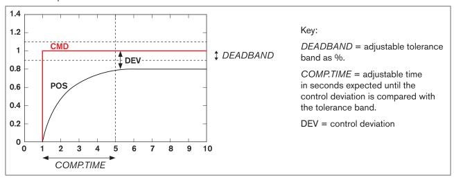
Figure 88: POS.MONITOR; schematic representation of position monitor
