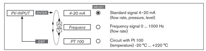
Figure 26: Operating structure PV-INPUT
