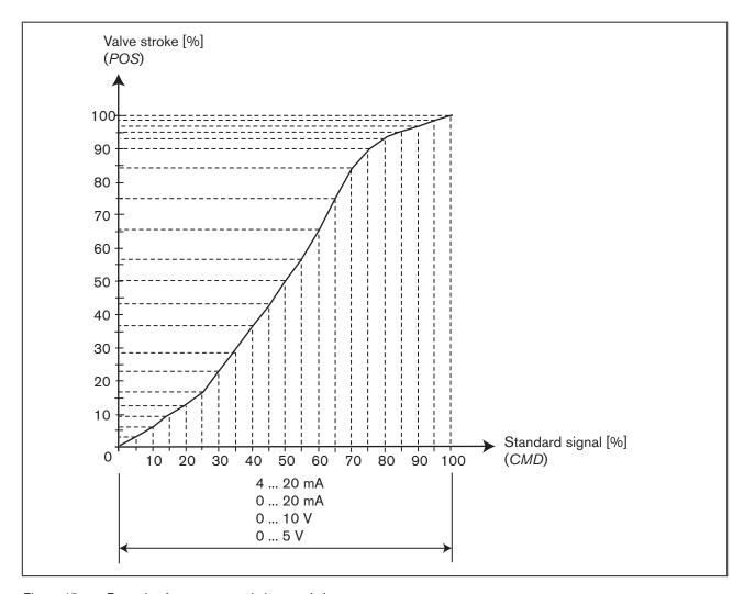
Figure 45: Example of a programmed characteristic
