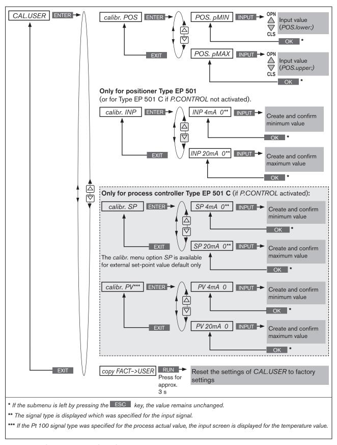
Figure 67: Operating structure CAL.USER
