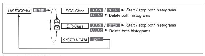
Figure 76: HISTOGRAM; operating structure
