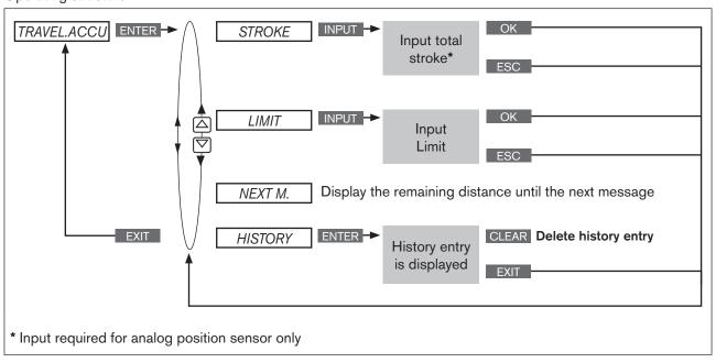
Figure 84: Operating structure TRAVEL.ACCU
