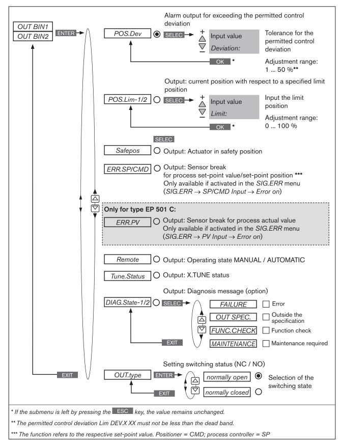
Figure 66: Operating structure OUTPUT-BIN1/BIN2
