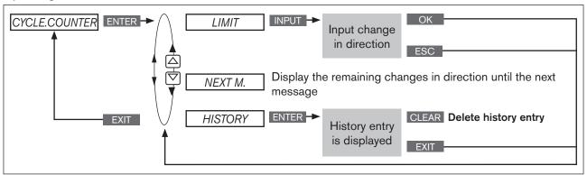
Figure 85: Operating structure CYCLE.COUNTER
