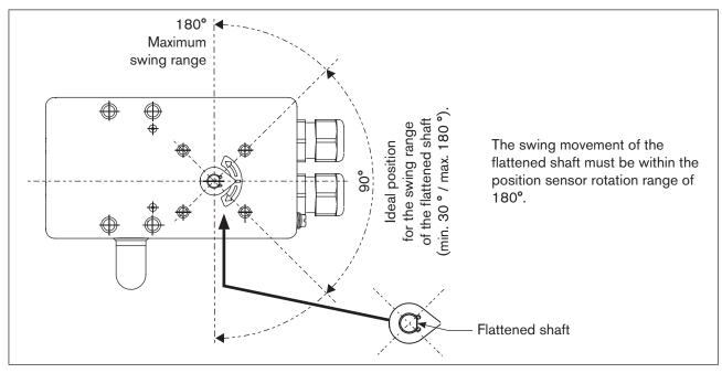
Figure 13: Rotation range / anti-twist safeguard
