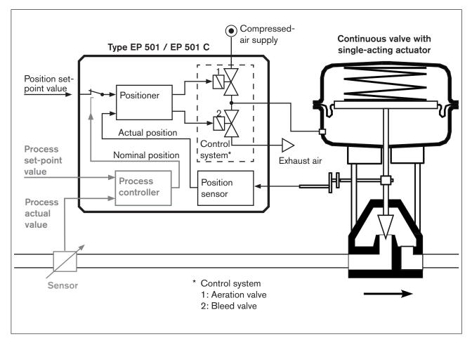
Figure 2: Structure, positioner Type EP 501 / process controller EP 501 C
