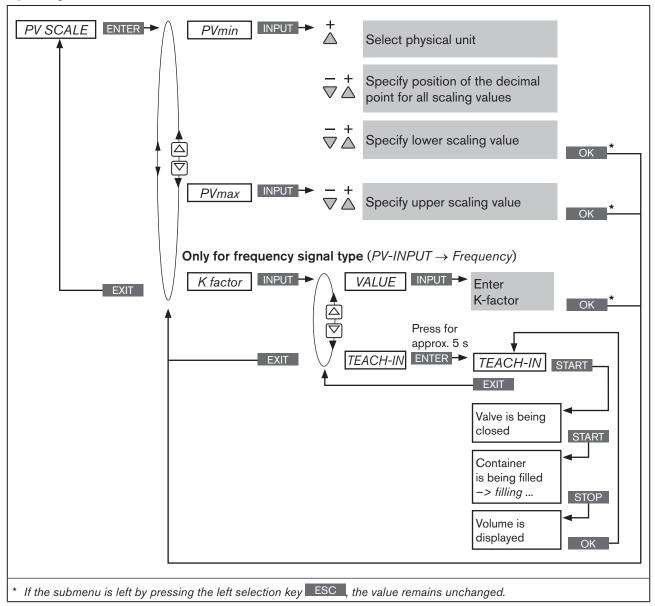
Figure 27: Operating structure PV-SCALE
