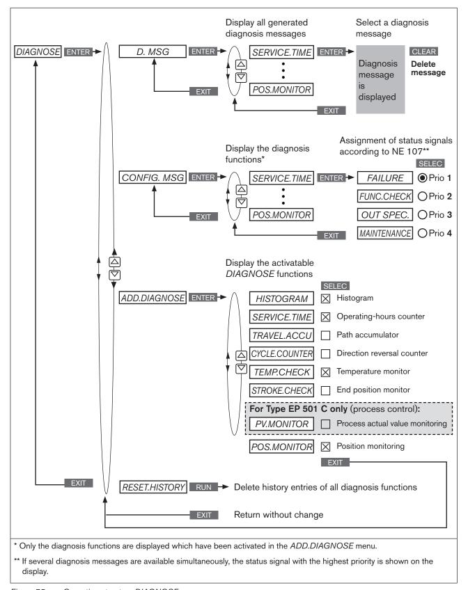
Figure 75: Operating structure DIAGNOSE
