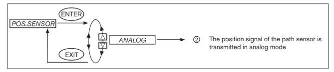
Figure 71: Operating structure POS.SENSOR
