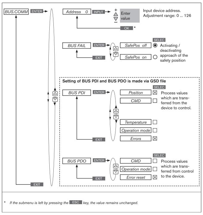
Figure 108: Operating structure - BUS.COMM; PROFIBUS DP
