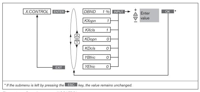
Figure 58: Operating structure X.CONTROL
