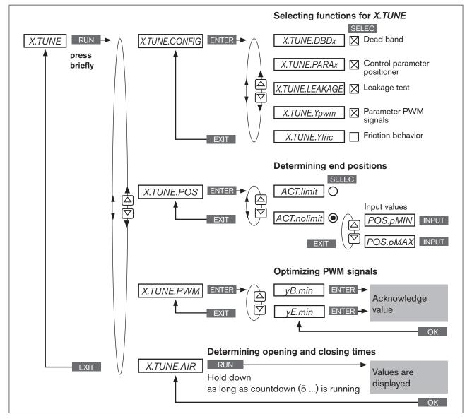
Figure 90: Operating structure for the manual configuration of X.TUNE
