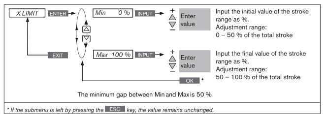
Figure 54: Operating structure X.LIMIT
