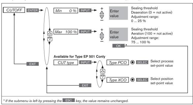
Figure 46: Operating structure CUTOFF
