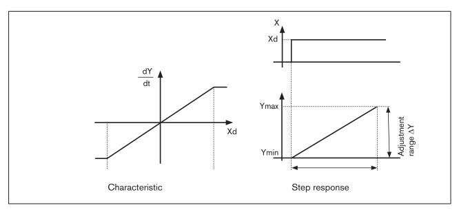
Figure 112: Characteristic and step response of the I portion of a PID controller
