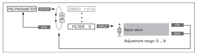
Figure 39: Operating structure FILTER; filtering of the process actual value input
