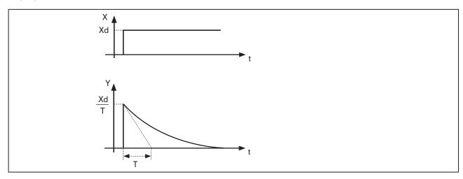
Figure 115: Characteristic of superposition of P, I and DT Portions
