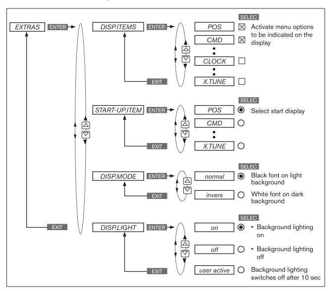
Figure 70: Operating structure EXTRAS
