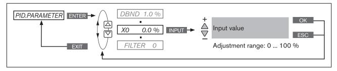
Figure 38: Operating structure X0; operating point
