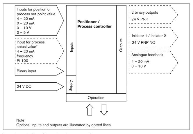
Figure 7: Interfaces of the positioner / process controller
