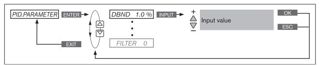
Figure 33: Operating structure DBND; insensitivity range
