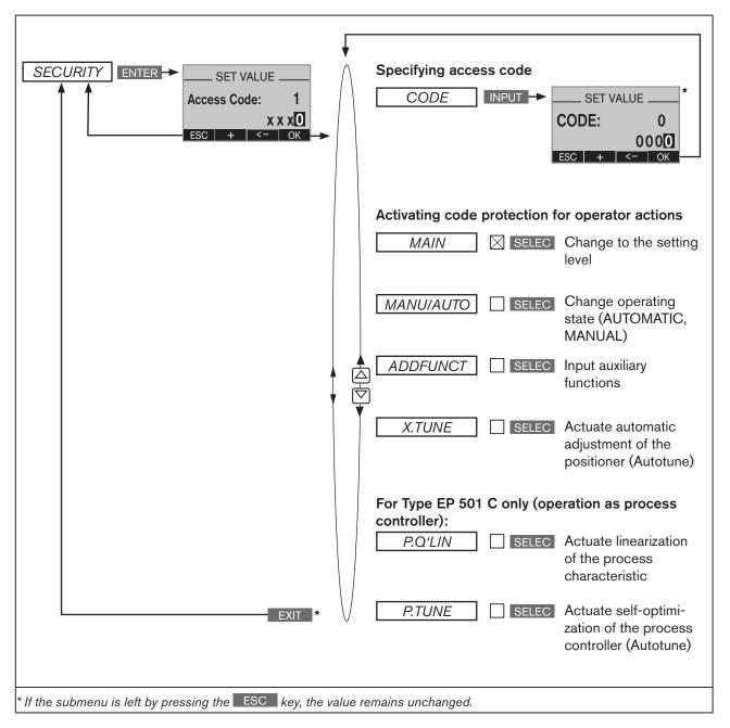
Figure 60: Operating structure SECURITY
