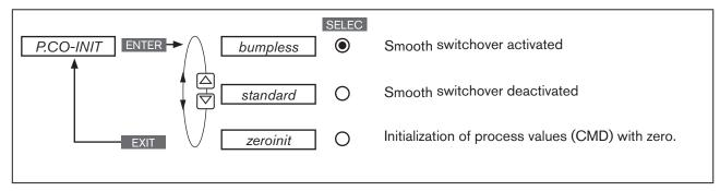
Figure 32: Operating structure P.CO-INIT
