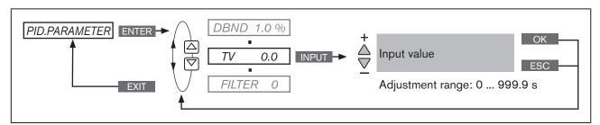
Figure 37: Operating structure TV; hold-back time
