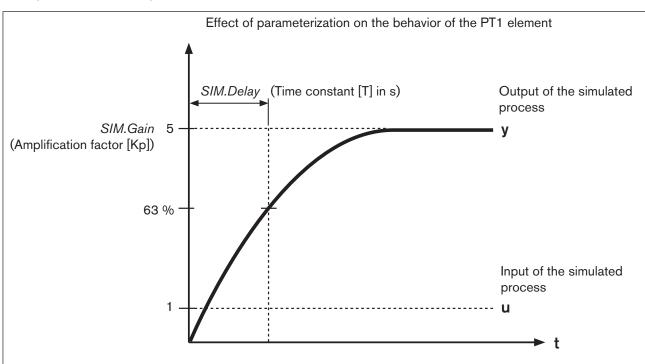
Figure 73: Example of a simulated process. Behavior of the PT1 element
