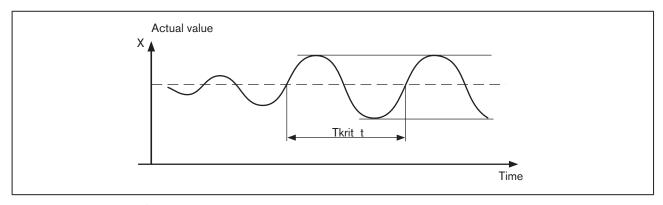
Figure 117: Progress of the control variable PID
