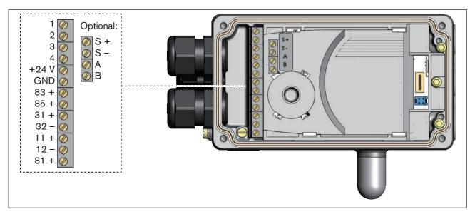
Figure 17: Designation of the screw-type terminals
