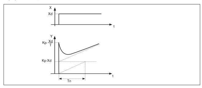
Figure 116: Characteristic of step response of the real PID controller; adjustment rules for PID controllers
