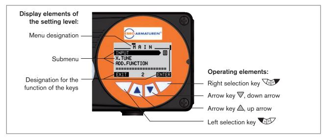
Figure 20: Display and operating elements of the setting level
