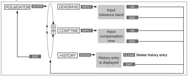
Figure 89: Operating structure POS.MONITOR
