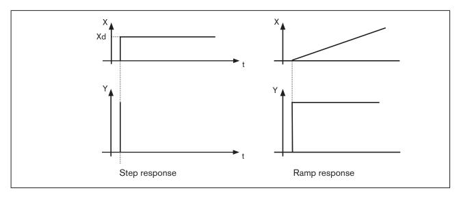
Figure 113: Characteristic and step response of the D portion of a PID controller
