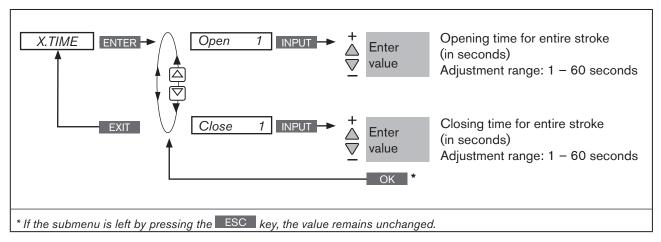
Figure 56: Operating structure X.TIME
