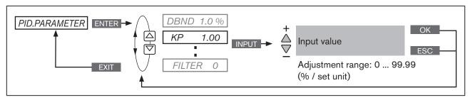
Figure 35: Operating structure KP; amplification factor
