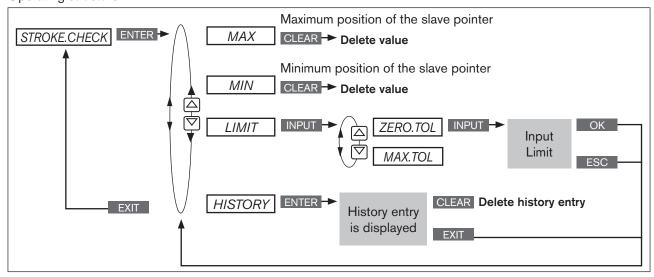
Figure 87: Operating structure STROKE.CHECK
