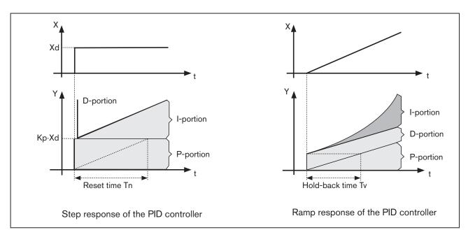
Figure 114: Characteristic of step response and ramp response of PID controller
