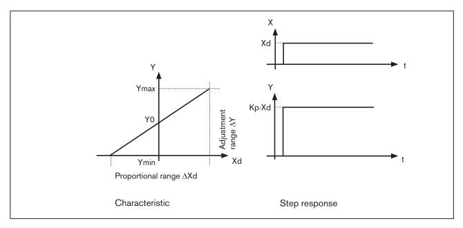
Figure 111: Characteristic and step response of the P portion of a PID controller
