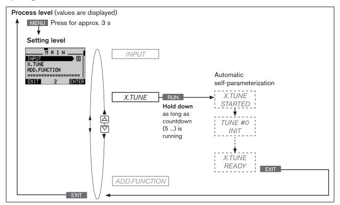
Figure 24: Operating structure X.TUNE
