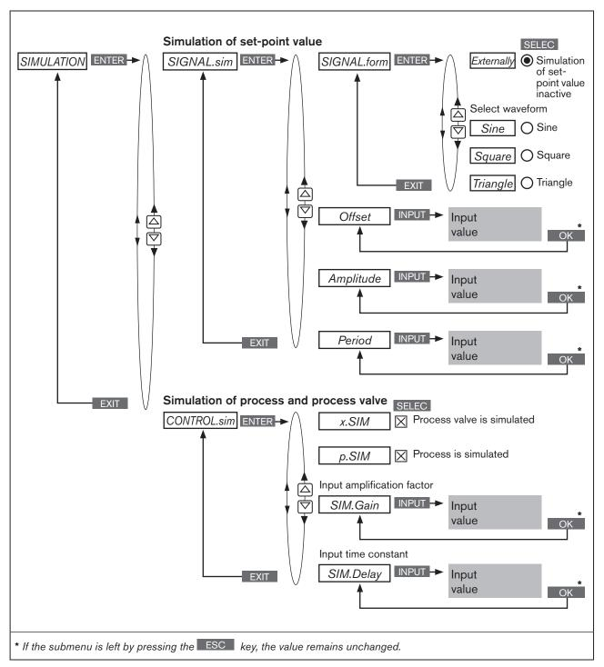
Figure 72: Operating structure SIMULATION
