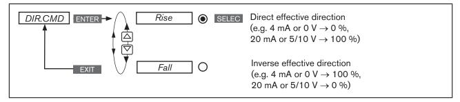
Figure 48: Operating structure DIR.CMD
