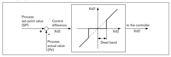
Figure 34: Diagram DBND; insensitivity range for process control
