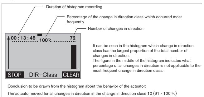
Figure 82: DIR class; histogram of the dwell time density for sinusoidal progression of the actuator position
