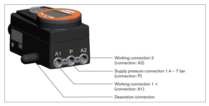
Figure 16: Fluid installation / Location of the connections
