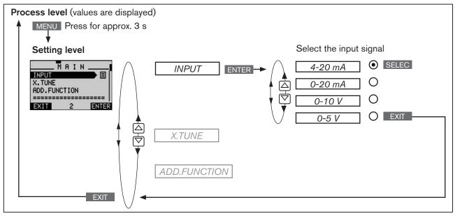
Figure 23: Operating structure INPUT
