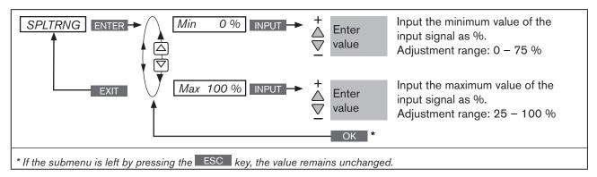
Figure 52: Operating structure SPLTRNG
