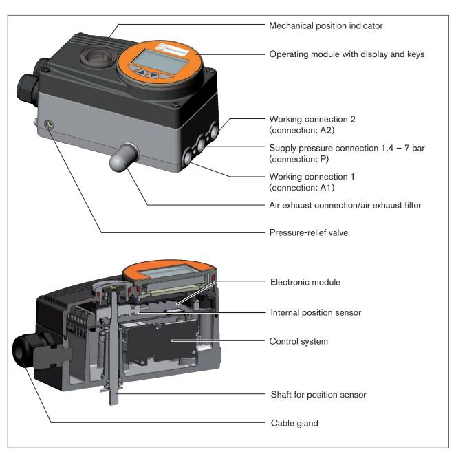
Figure 1: Structure, Type EP 501
