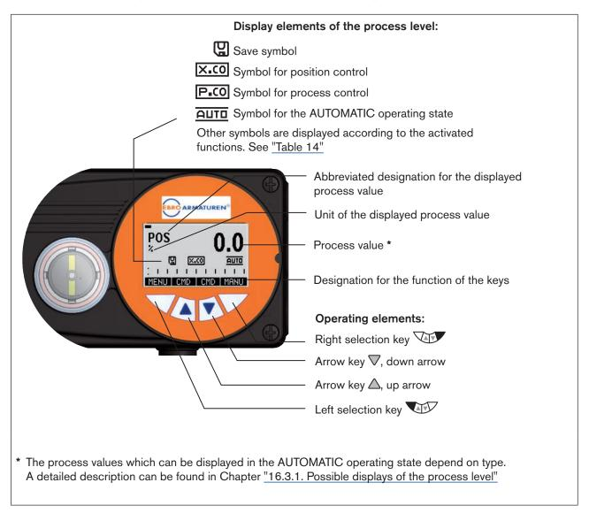
Figure 19: Display and operating elements of the process level
