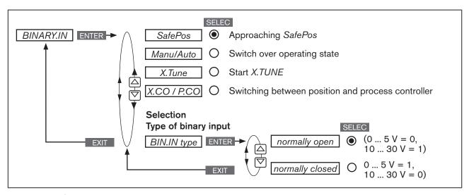
Figure 63: Operating structure BINARY.IN
