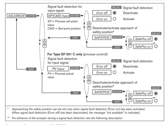
Figure 62: Operating structure SIG-ERROR
