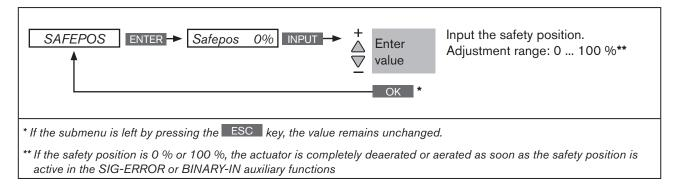
Figure 61: Operating structure SAFEPOS
