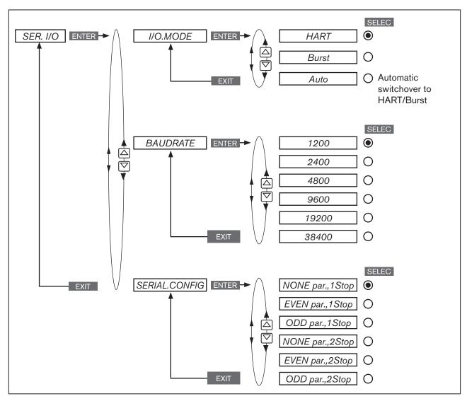
Figure 69: Operating structure SER. I\O
