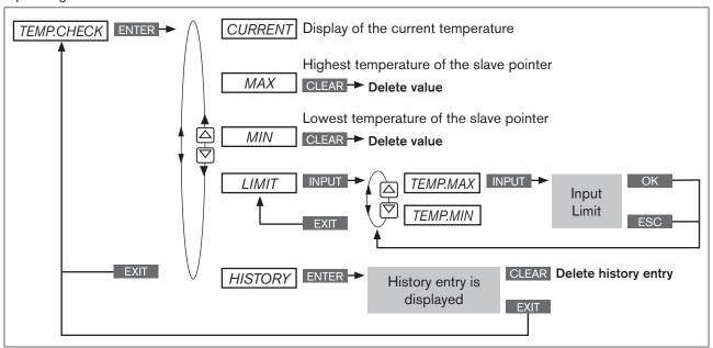
Figure 86: Operating structure TEMP.CHECK
