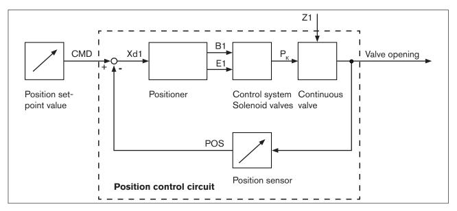
Figure 3: Position control circuit in Type EP 501
