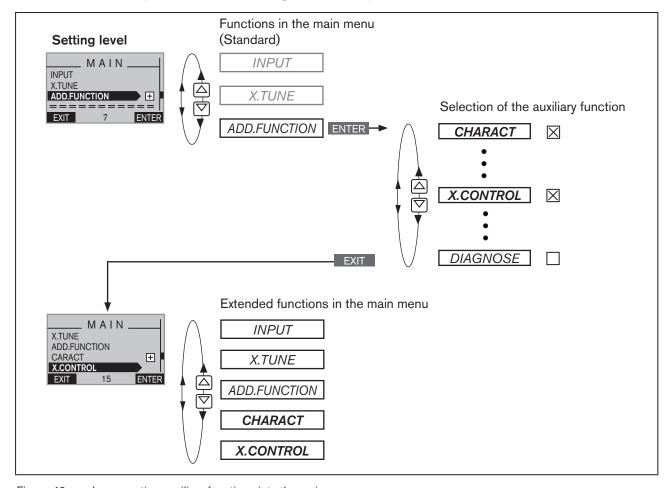
Figure 40: Incorporating auxiliary functions into the main menu
