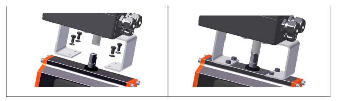
Figure 15: Rotary actuator attachment
