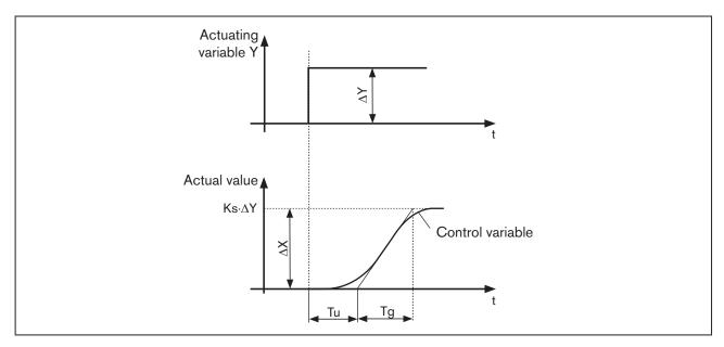
Figure 118: Progress of the control variable, actuating variable jump
